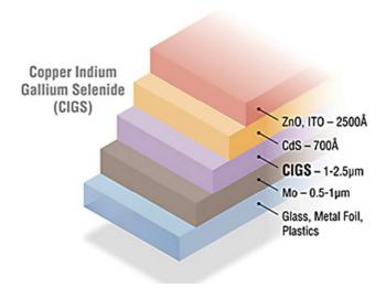
Fig. 7. Graphic showing the five layers that comprise CIGS solar cells.
