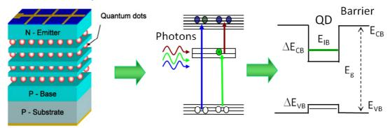
Schematic of operating principle and energy band diagram of proposed III-(As, SB)solar cell
