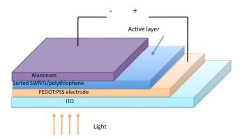
Fig. 10. Structure of carbon nanotubes based solar cells.
