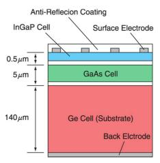
Fig. 9. Cross-sectional diagram of InGaP/GaAs/Ge.
