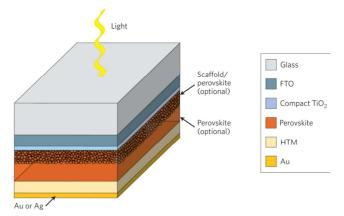
Fig. 16. Perovskite solar cell structure.
