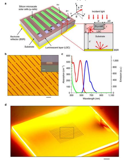
Fig. 11. A luminescent concentrator system with an array of surface-embedded monocrystalline silicon solar  $\mu$ -cells (a) Schematic illustration of a device, consisting of an array of solar microcells ( $\mu$ -cells), a luminescent layer (LSC layer), a supporting, transparent substrate and a BSR. The inset on the right shows a cross sectional view, with key.
