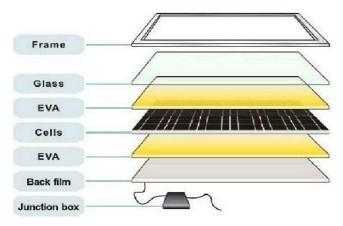
Fig. 13. Monocrystalline solar cell structure.
