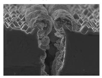
Fig. 4. Cross section of a partially plated laser groove.
