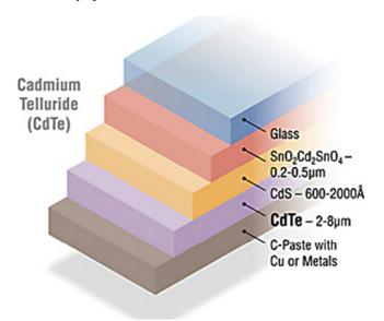
Fig. 5. Graphic showing the five layers that comprise CdTe solar cells.
