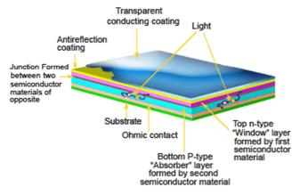
Fig. 21. Structure of thin film solar cells.
