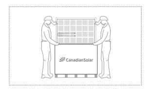
Do not stand, step, walk and / or jump on modules under any circumstances. Localized heavy loads may cause severe micro-cracks at cell level, which in turn may compromise module reliability.
